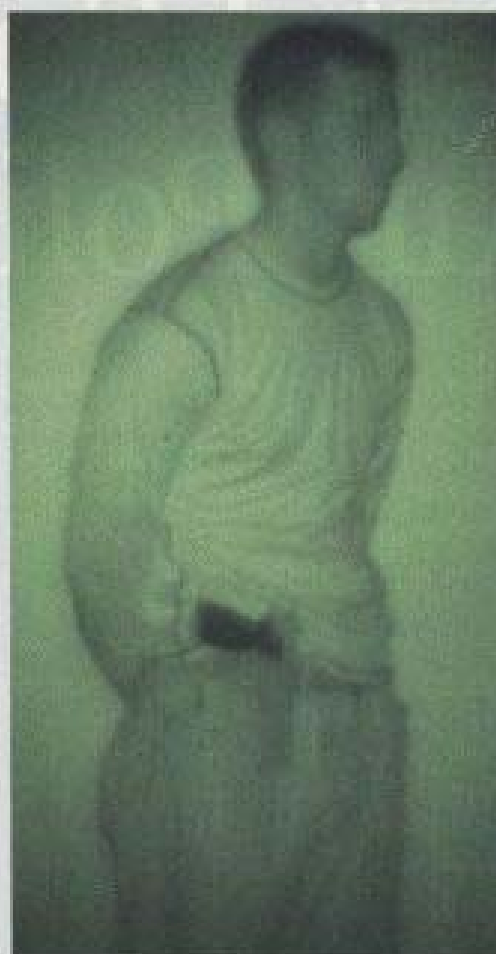
The use of an infrared illuminator makes all the difference. Under dark (no moon) lighting conditions with an IR, both the Gen 1 and Gen 2 (shown) devices picked up the pistol.
